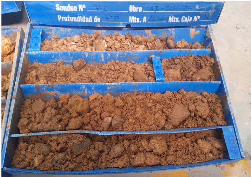
Testigo del sondeo P1 (7,40 – 10,00m)
